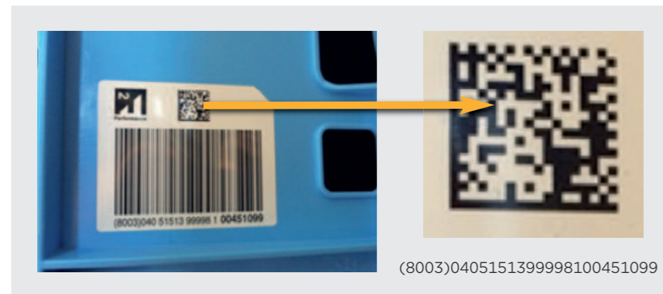
Figure 4 – Example for a meat crate containing a GRAI encoded in a GS1 DataMatrix
