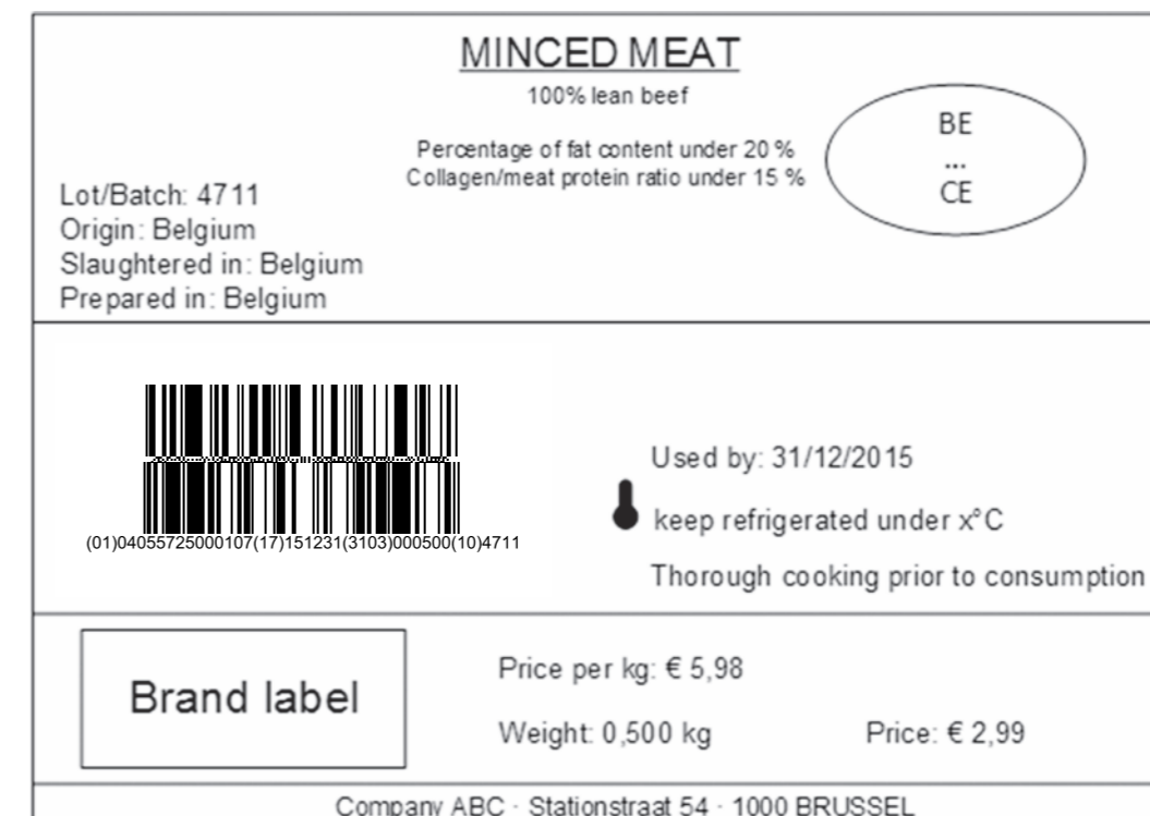
Figure 7 – Label for pre-packed variable/fixed weight product sold at PoS with GS1 DataBar
